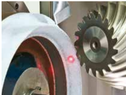
With the help of precise laser alignment, the operator can more accurately position the coolant header for optimum coolant flow.
