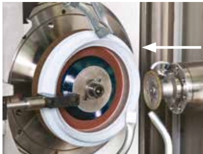
The dressing unit has been designed so that it telescopes forward into the work area for dressing, but then completely retracts flush with the guarding during the grinding operation.
