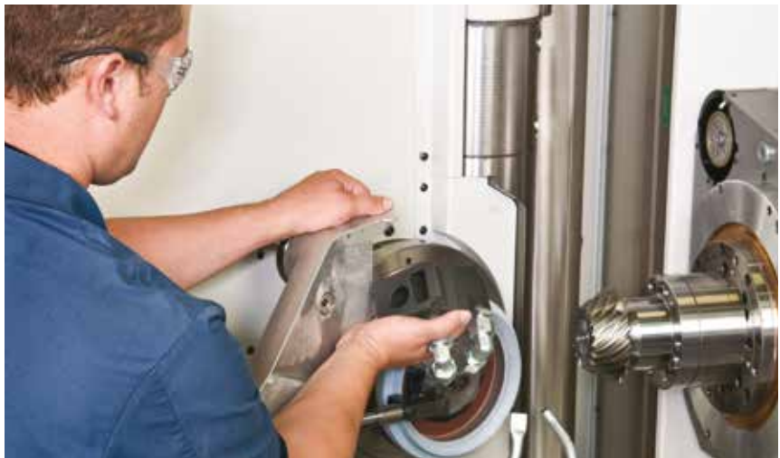
The new quick-change coolant header enables the operator to quickly and efficiently change and re-position the headers for each new job.
