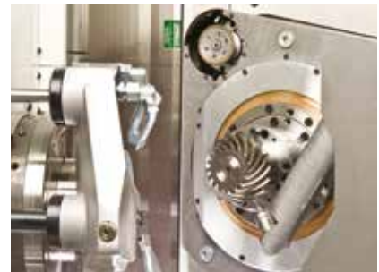
The Automatic Stock Divider features a very stiff design for greater reliability, and operates simultaneously with wheel dressing to reduce non-productive time.
