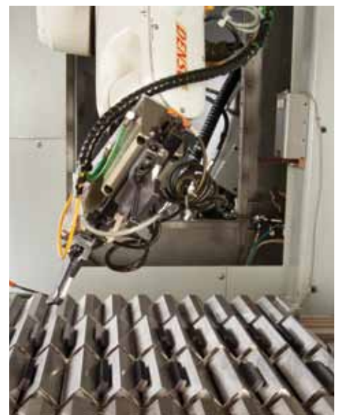
Gantry loader takes stick blade from the tilt station and transfers it to the grinding area of the machine.
