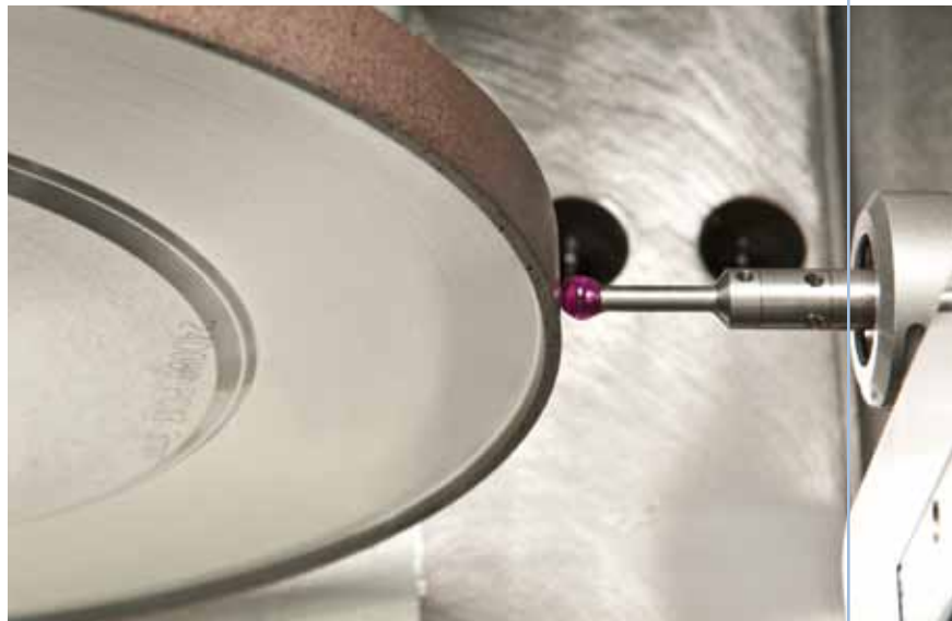
Grinding wheel probing.
