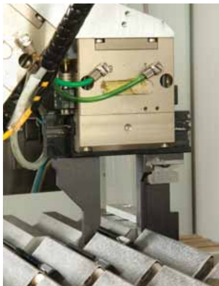
Robot transfers stick blades to the tilt station.
