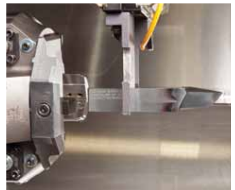
Gantry loader takes stick blade from the tilt station and transfers it to the grinding area of the machine.
